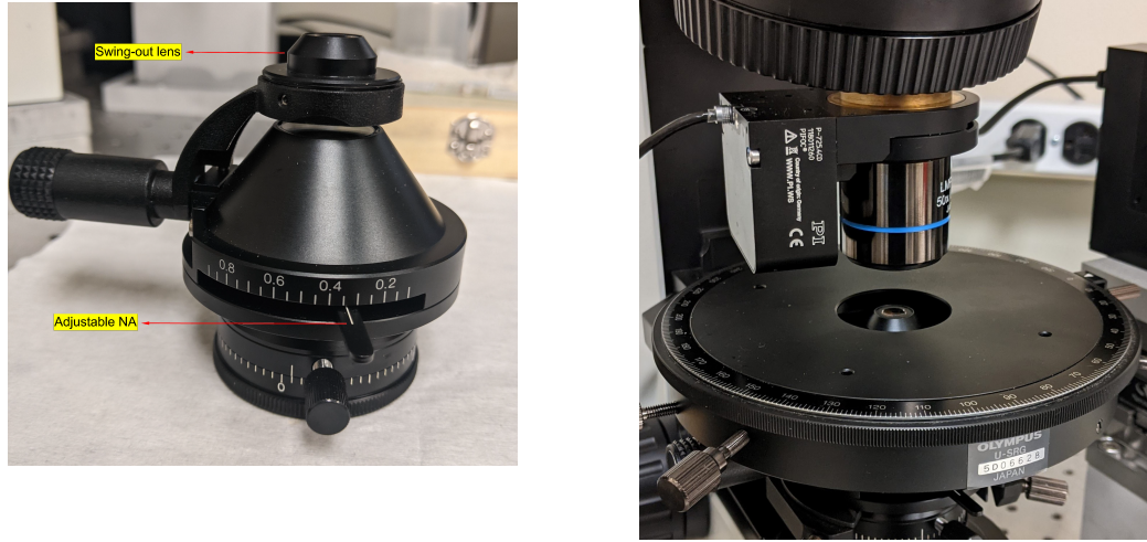
Figure 4.3: Left: Olympus U-SC swing out achromatic condenser with adjustable NA setting (used for disk illumination). Right: Photograph of the Olympus UmPlanFI 50x objective used in the experiments (The objective is attached to the POS).
