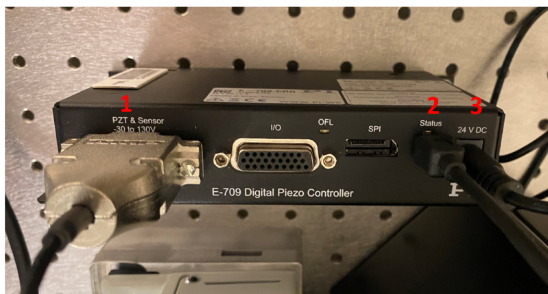
Figure A.9: E-709 Piezo Controller. (1) Fiber optic connection to translator; (2) USB connection to computer; (3) Power connection to wall power supply.
