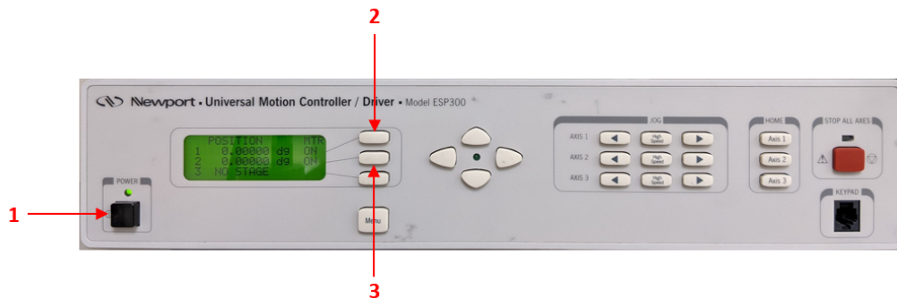
Figure A.8: ESP300 motion controller. (1) Power button on. (2) Axis 1 on. (3) Axis 2 on.
