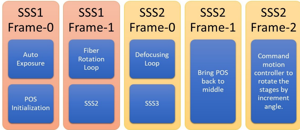
Figure 3.11: Summary of operations performed by each frame in SSS1 and SSS2.
