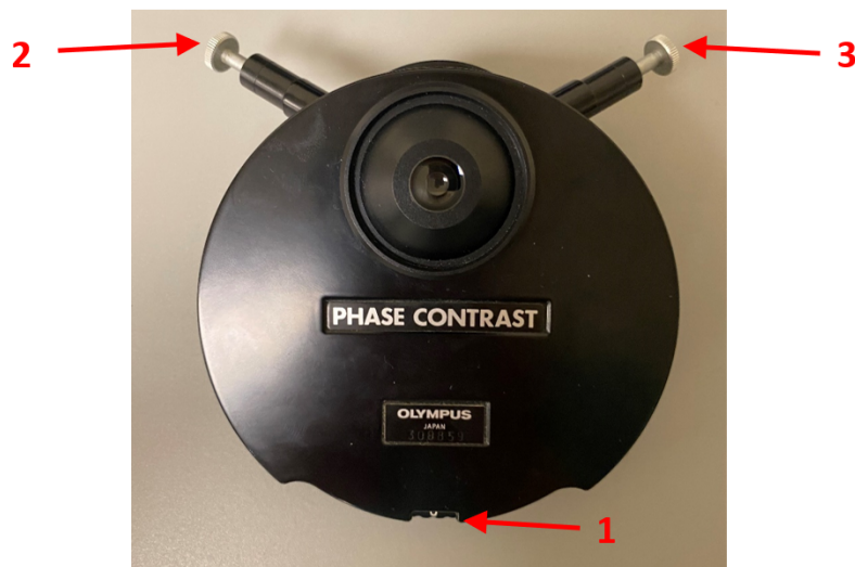
Figure A.19: U-PCD2 Phase contrast condenser. (1) Annulus selector. (2) & (3) annulus centering knobs.
