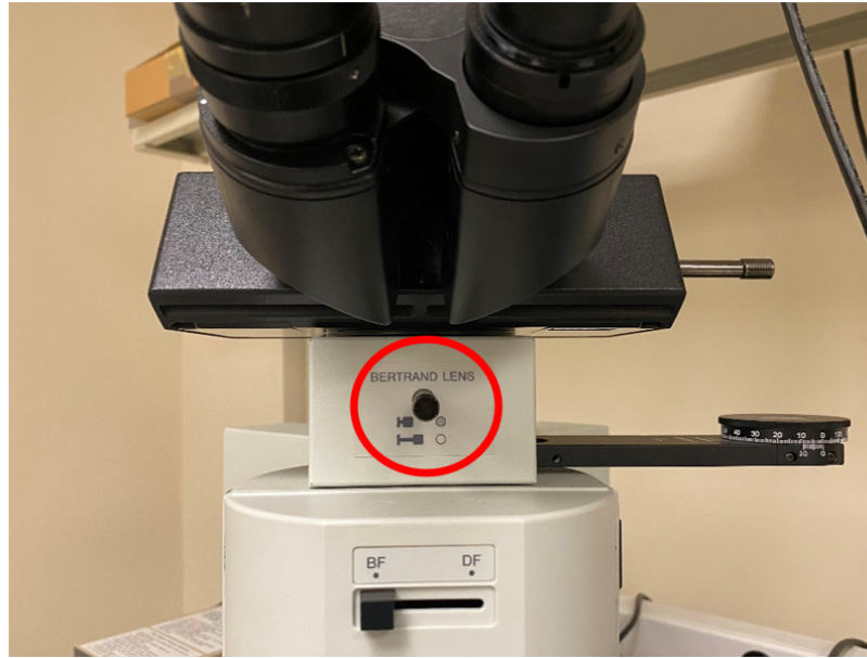
Figure A.21: Bertrand lens selector knob. Pushed into the microscope Bertrand lens is selected, pulled out of the microscope the Bertrand lens is omitted.
