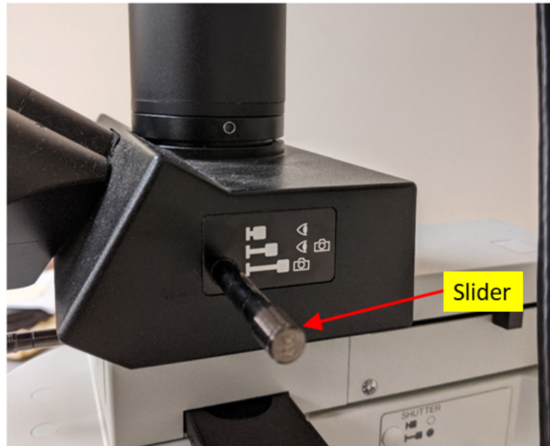
Figure A.5: Slider (showed by red arrow) to set the beam splitter.
