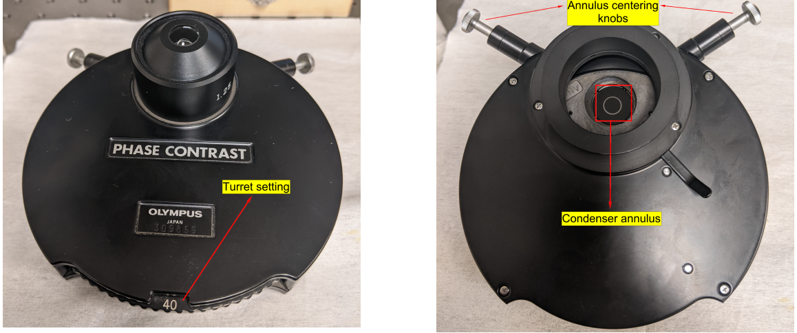
Figure 4.4: Olympus U-PCD2 phase contrast condenser. Left: top face of the condenser with turret setting. Right: bottom face of the condenser with annulus centering knobs and condenser annulus highlighted in red (used for annular illumination).
