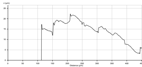
Figure 4.31: Edge of stereolithography part, captured at 20x
