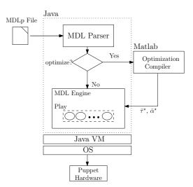
Fig. 6. The puppet system software architecture.
