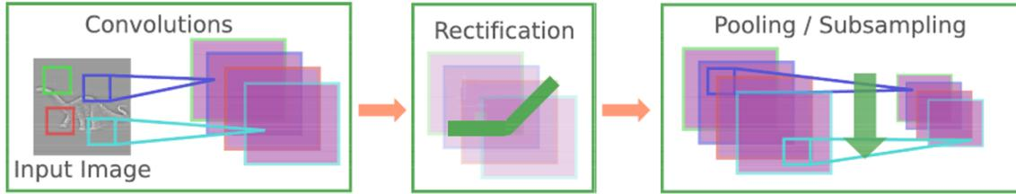
Figure 5.22: Notional convolutional layers including the convolution, rectification, and pooling layers. Modified from [178].
