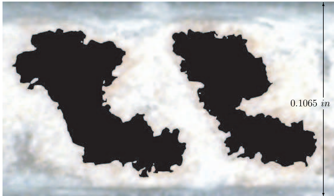
Figure 26: Color similarity algorithms used to identify and segment Jute yarns from background
