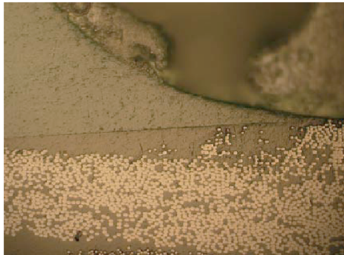
Figure 64: Photograph showing disbonding at the adhesive interface in short bondline fabric specimen #4 (200X)
