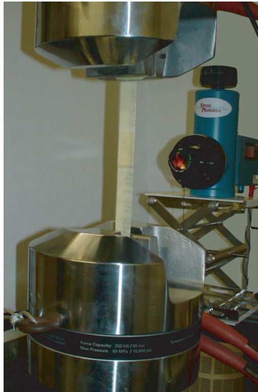
Figure 49: Infrared camera and the IR-TSA experimental setup
