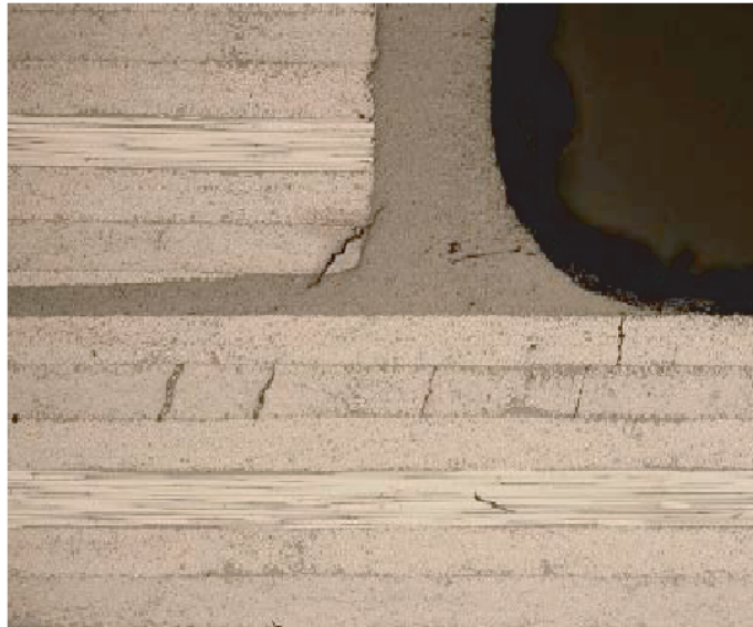
Figure 65: Photograph showing micro-cracking in short bond line uni-tape specimen #5 (50X) corresponding to IR-TSA in Figure 60.
