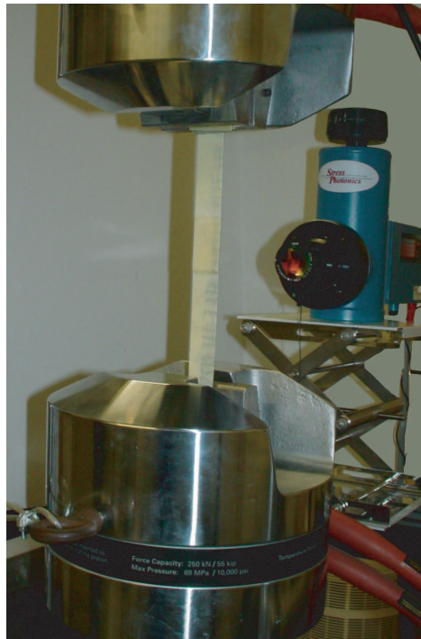
Figure 66: Fatigue Test Setup for S2-glass/E733FR Single Lap Joints
