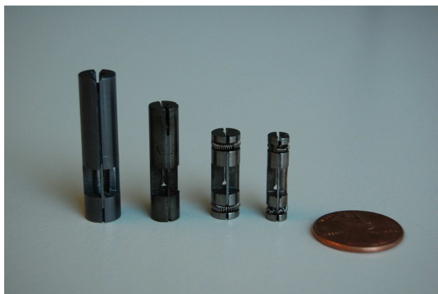
Figure 2.6: Blade-side view of the four BRIM designs, with a penny for scale. Left to right: MK2BRIM_138, MK2BRIM_276, MK3BRIM_276, MK3BRIM_414.
