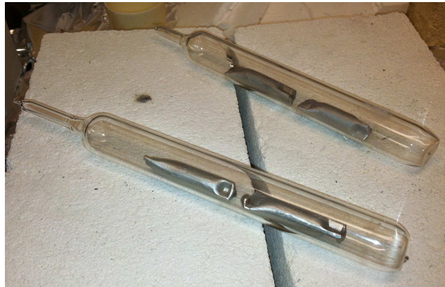
Figure 6.1: For \text{Sc}_{1-x}\text{M}_x\text{F}_3 syntheses, welded nickel (or copper) ampoules were sealed in evacuated fused quartz tubes. This figure shows two reaction vessels containing Ni ampoules prior to heating in a furnace for 72 h.
