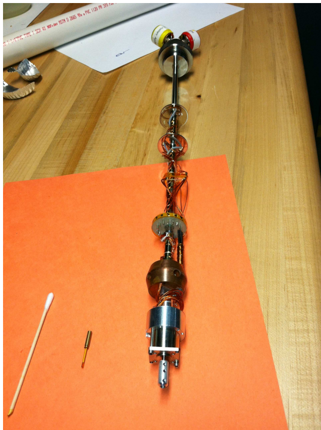
Figure 2.4: Helium cryostat sample stick used at beamline 11-BM-B of the Advanced Photon Source. The sample capillary, shown at left, is placed at the end of the stick at the bottom of the image.
