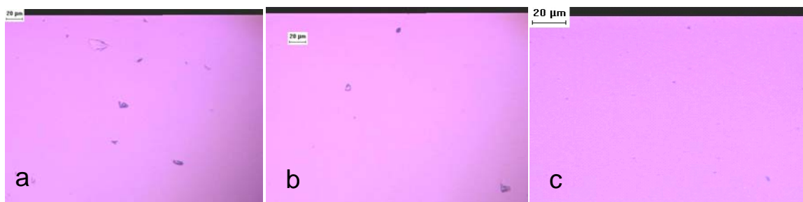
Figure 7-17: Photomicrographs of crystals of non-oxidized HGD obtained upon addition of the following solutions at 298 K (a) 20 mM \text{CaCl}_2 (b) 20 mM \text{CaCl}_2 and 100 mM NDSB-201 (c) 20 mM \text{CaCl}_2 and alpha A-crystallin. Crystals were obtained in every solution.
