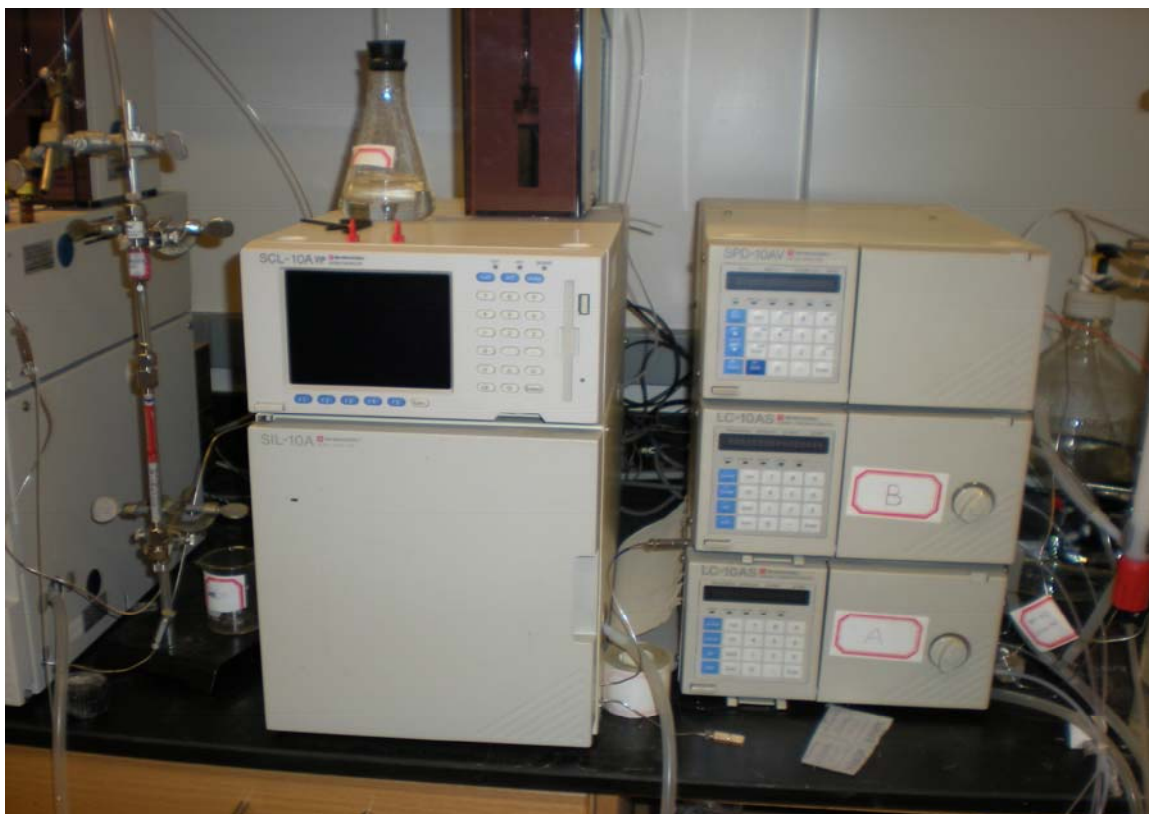
Figure B-2: Shimadzu system used for UV detection. The controller is on the left, and pumps A and B and the UV detector are on the right.
