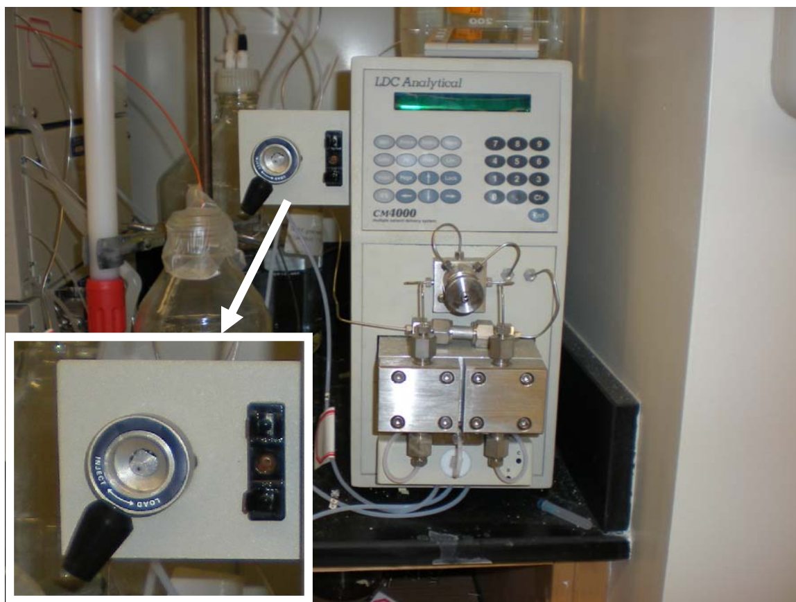
Figure B-1: The LDC Analytical Pump (CM4000) showing the injection valve in the "inject" position.
