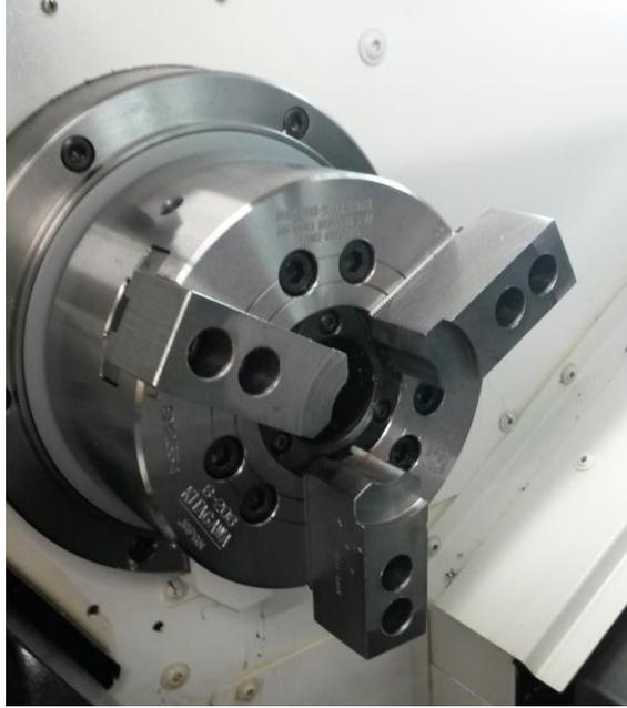
Figure 11. Softjaws for Yoyo Machining
