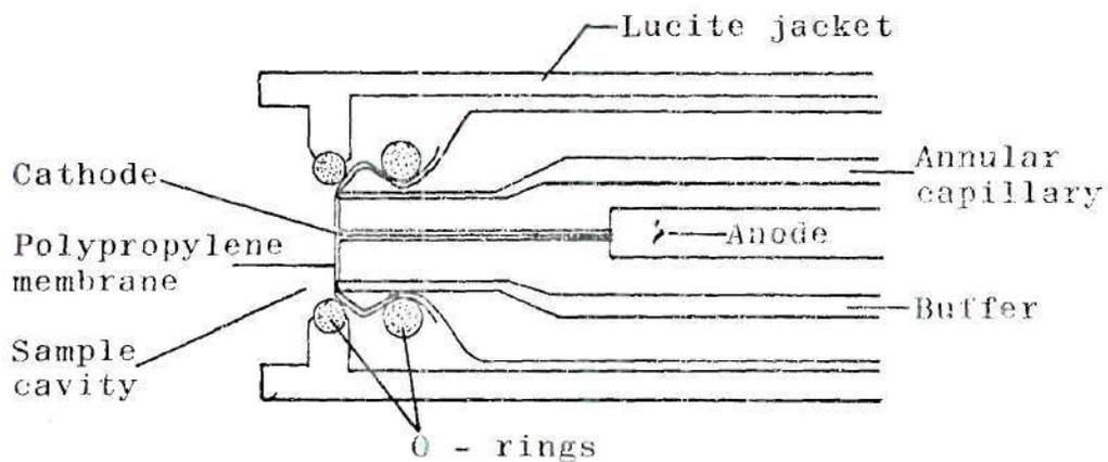
Figure 14. Cross Section of Carbon Dioxide and Oxygen Electrodes
