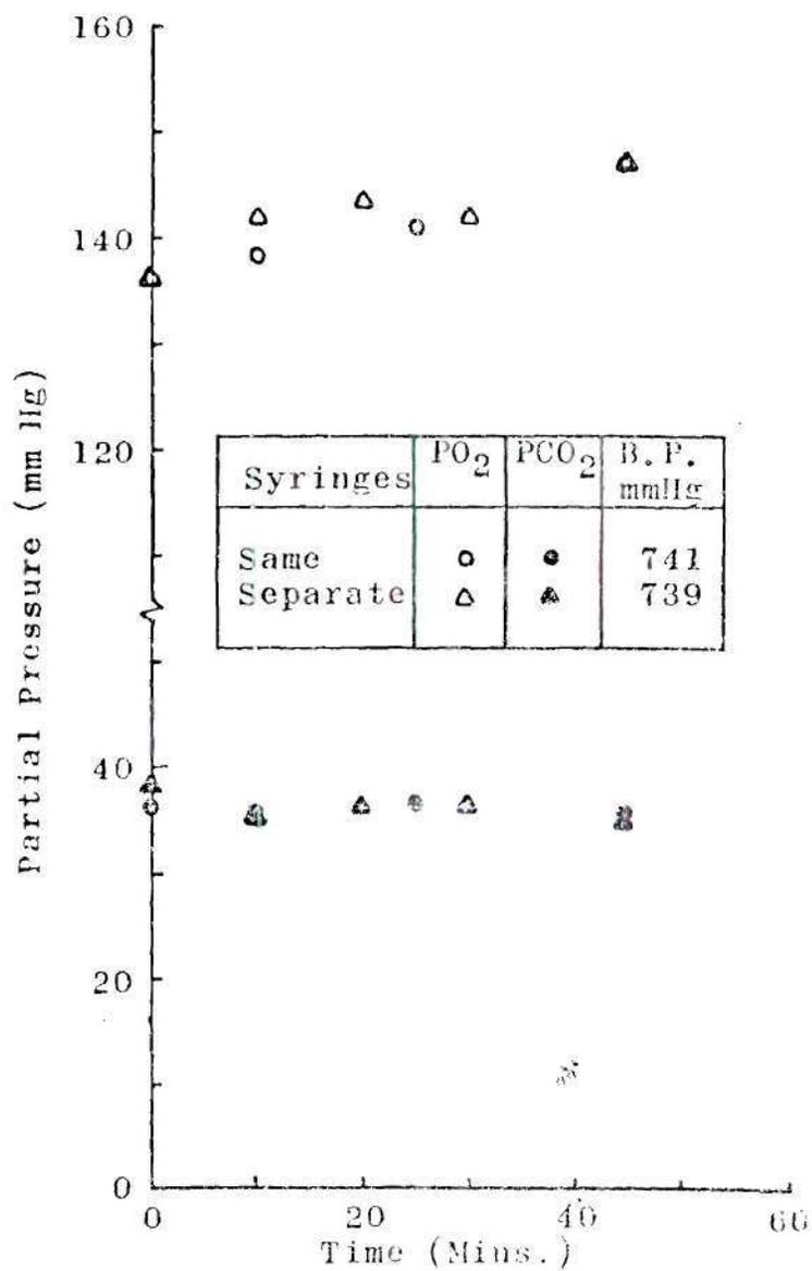
Figure 5. Partial Pressures of Oxygen and Carbon Dioxide vs. Storage Time for Blood Equilibrated with 5.1% CO<sub>2</sub>, 19.7% O<sub>2</sub> and Ice
