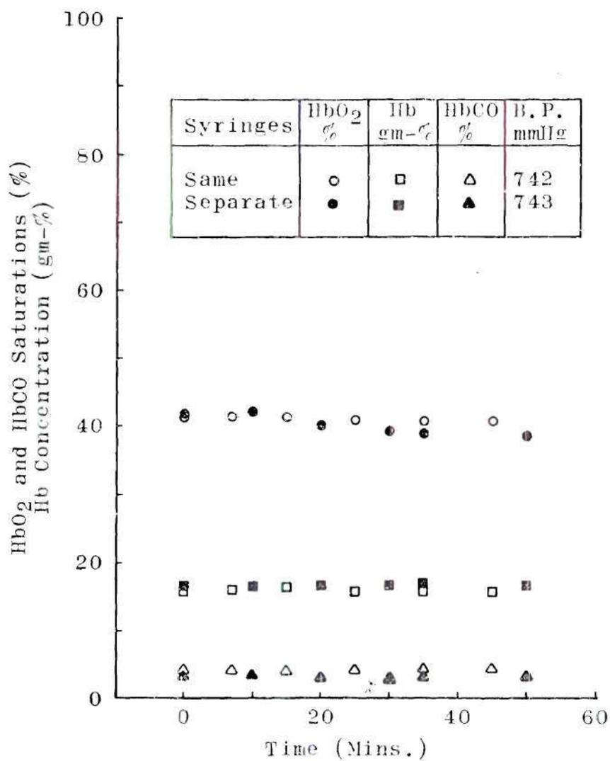
Figure 8. Concentrations vs. Storage Time for Blood Equilibrated with 5.3% CO<sub>2</sub>, 3.2% O<sub>2</sub> and Iced in Plastic Disposable Syringes
