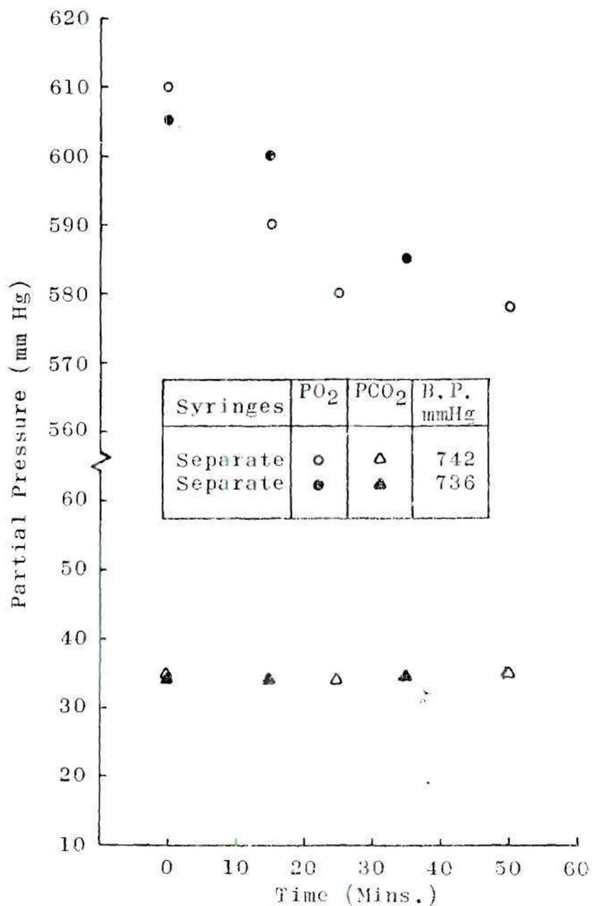
Figure 12. Oxygen and Carbon Dioxide Partial Pressures vs. Storage Time for Blood Equilibrated with 5.0% CO<sub>2</sub>, 95.0% O<sub>2</sub> and Iced in Plastic Disposable Syringes; IL-113 Used for Gas Analyses
