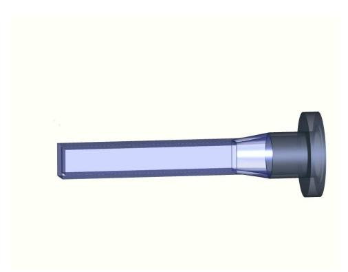
Figure 4.1: An AutoCAD drawing of the cell used for the experiments. The cell is made from quartz, with square cross section of 1". There is glass transition piece that takes the cell to a standard 2.75" CF vacuum connection, which connects to an ion pump.
