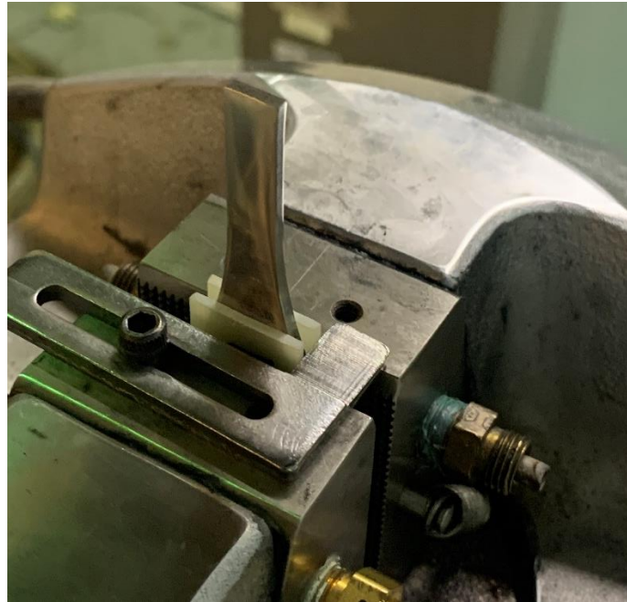
FIGURE 31: The fixture used to ensure fatigue specimens are horizontally aligned.
