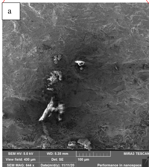
FIGURE 86: Nucleation site of specimen 5-9 (small z, polished, 168.8 MPa).
