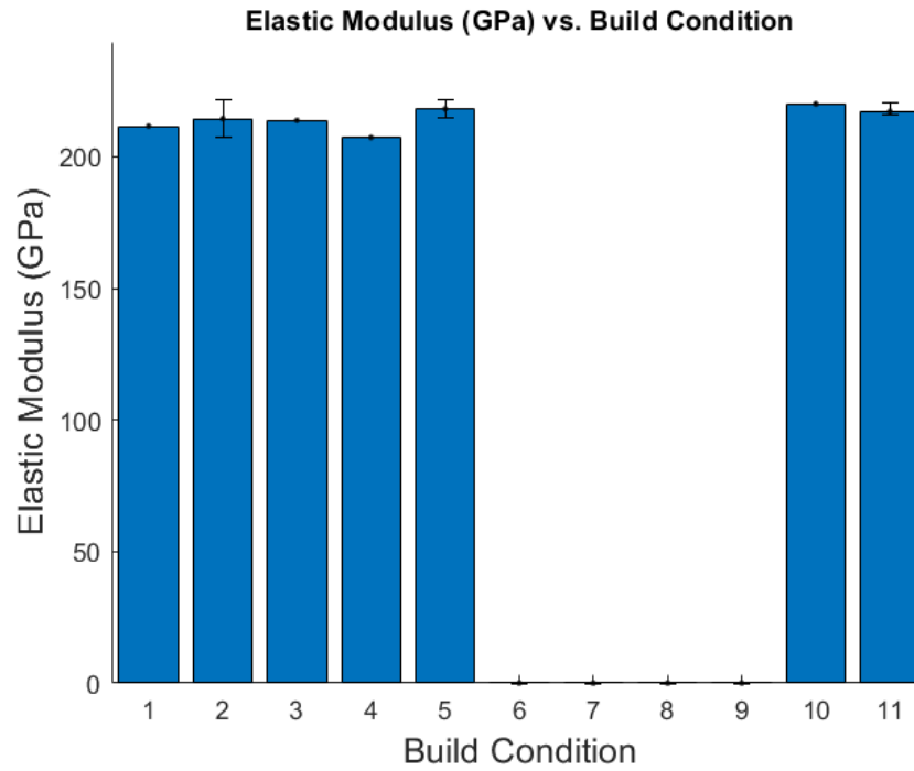
FIGURE 54: Elastic modulus vs. build condition for xy tensile specimens.
