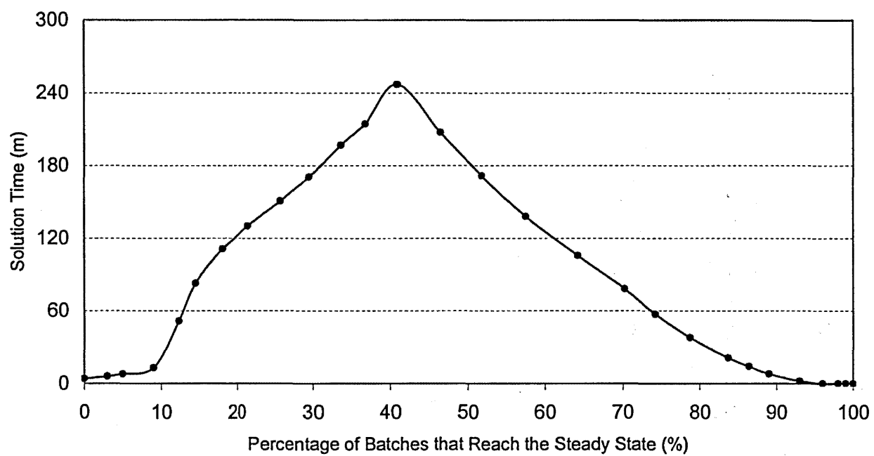
Figure 5.4 Solution time corresponding to percentage of batches that reach the steady state
