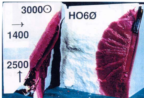
Figure 1.23 Fracture surface with steps at wellbore inclined at 60^\circ with respect to the least principal stress [ Abass et al., 1996 ]. The numbers shown indicate confining principal stress in pounds per square inch (psi).
