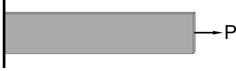
Figure 21: Composite Strip with k_3 = 0 , subjected to a tip force P as shown
