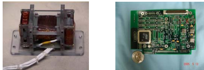
Figure 9. Fluxgate Sensor (left) and Electronics (right)
