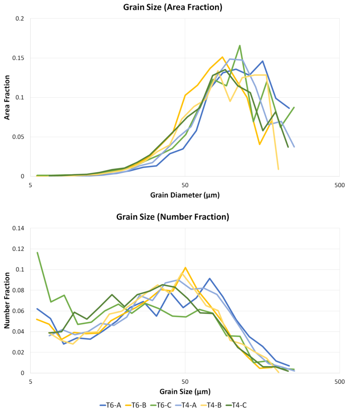
Figure 38. Grain size distribution plotted against area fraction (top) and number fraction (bottom). Grains whose diameters were less than 5 and 6 \mu\text{m} in the T6 and T4 EBSD scans, respectively, were excluded from the analysis. Blue, yellow, and green represent samples with compositions A, B, and C, respectively.
