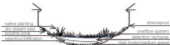
Utilizing rain gardens to filter and hold water
