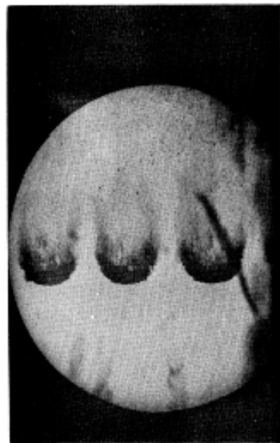
Shadow Photograph of 780\mu Waterdrops M_s = 1.54 T = 45\ \mu\text{-sec} After Shock Passage
