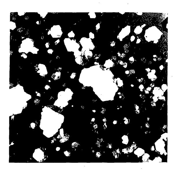
1819-64 Premax Clay, 79.9% Solids Mixed with a Cowles Dissolver for 10 Minutes 22,000X
