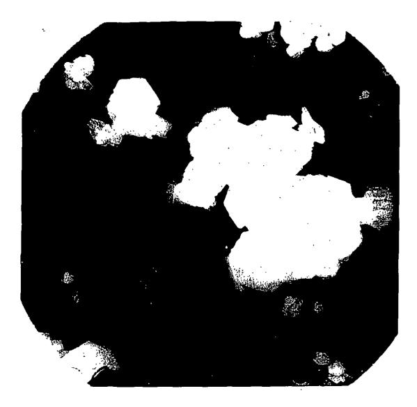
1679-153-1 Premax Clay, 69.68 Solids Mixed for 5 Minutes in Kady Mill, 3000 r.s.m. 22,0005
