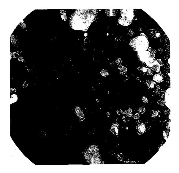
1679-153-6 Premax Clay, 69.65 Solids Mixed for 30 Minutes in Kady Mill 22,000%
