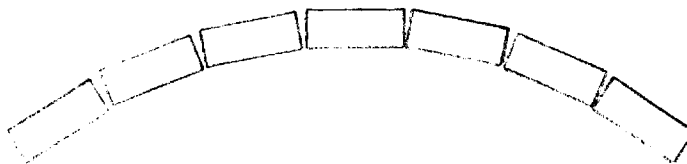
Figure 3. Cylindrical Array Composed of Broadwall Slots in Rectangular Waveguide.
