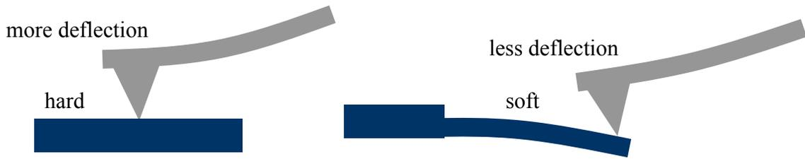
**Figure 2-7,** measurement of spring constant of a thermal cantilever
