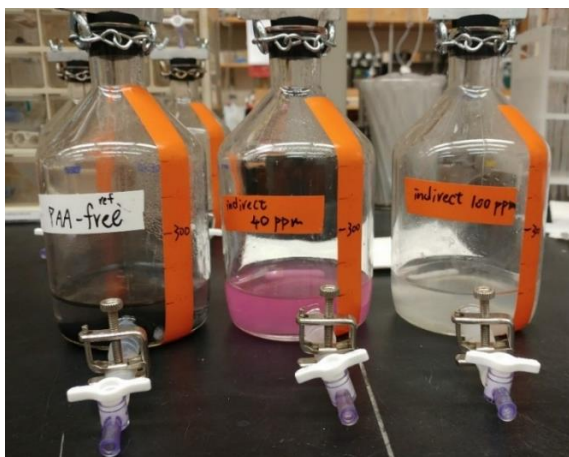
Figure 4.3. Color of the anaerobic culture medium of the reference (PAA-free), pre-decomposed 40 mg/L PAA, and pre-decomposed 100 mg/L PAA series (from left to right).
