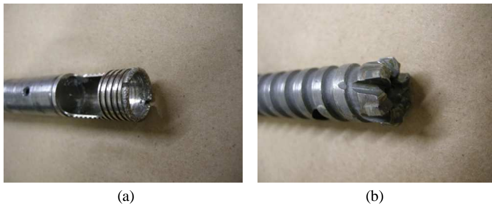
Figure 3.2 Borehole drilling tools (a) diamond core bit and (b) rebar-cutter.
