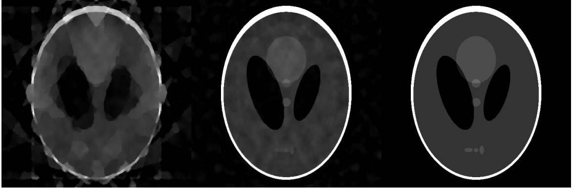
Figure 3.10: Recovered CT images (using first-order primal-dual) from Figure 3.8. The original image is given on the right hand side for comparison. The parameters for this experiment were \lambda = 10^3, \beta = 100 and the number of iterations were T = 2500 .
