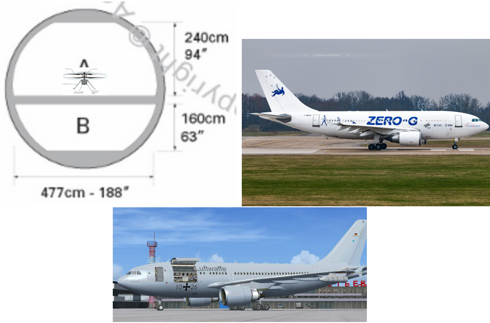
Figure 5: Left: Mars helicopter in A310 aircraft. Relative dimensions are approximate. Right: ESA A310 zero- g aircraft. Doors are those of a standard commercial jet. Bottom: A310 cargo aircraft with large cargo door.
