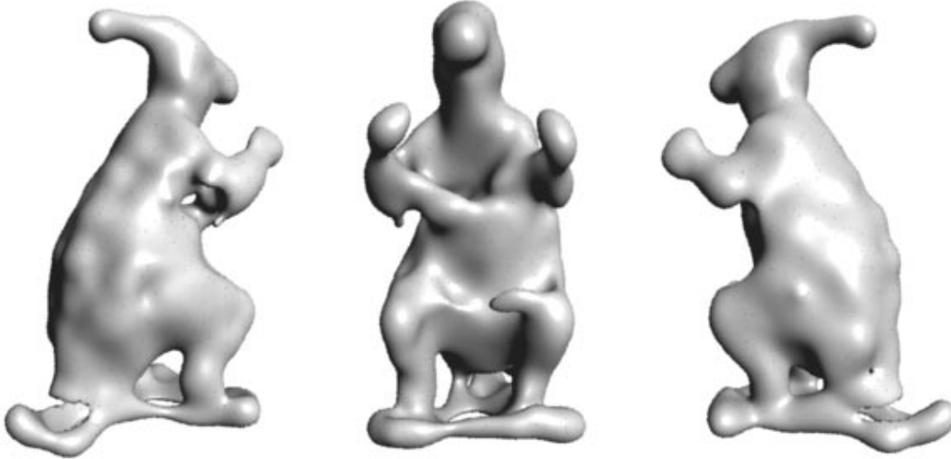
Fig. 5. The reconstruction is a variational implicit surface generated using the basis, \phi(r) = |r|^3 and \lambda = 0.001 for surface constraints. The data set is the same as that of Figure 3.
