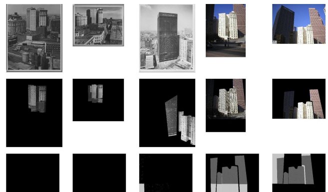
Figure 2: First row: input ordered images. Second row: visibility test through time and space. Third row: weighted mask on temporal distance warped to final view (brighter pixels have higher weights). The result of blending all textures weighted based on time is shown in Figure 1(d).
