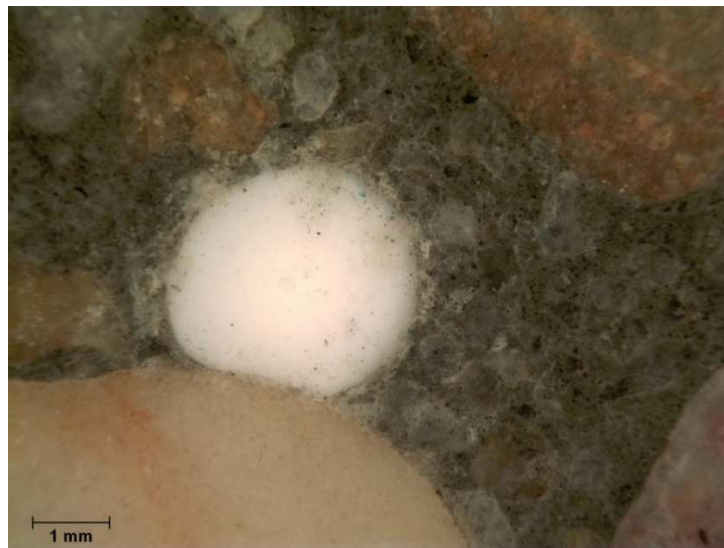
Figure 21. ASR gel in the freshly cut section of a concrete prism exposed to ASTM C1293 condition for more than one year.
