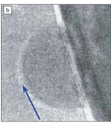
Figure 1. Large depression of the eutectic temperature of a nanometer-sized Sn-In alloy particle. (a) As-produced Sn-In alloy particle in a state of a solid solution, (b) the same particle, which underwent a melting transition by additional alloying of In. During the experiment, the temperature of the substrate was kept at room temperature (from Reference 2). Subscripted numbers in plane spacing values indicate uncertainty in that decimal space.
