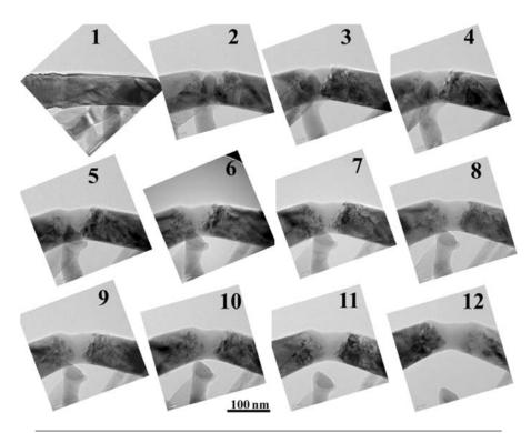
Figure 4. A series of transmission electron microscopy (TEM) images showing the bent SiC NWs from elastic (1) to plastic (2) and the large strain plasticity through 3 to 12. An amorphous character was directly observed in 3 and 12. The amorphous region shows transparent contrast in the middle, which is distinctive from the crystalline regions. (Image courtesy of X.D. Han and Z. Zhang, from Reference 10).
