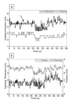
Figure 7. (a) Graphs showing the positions of the disordered (top) and ordered (bottom) sides of the diffuse interphase boundary in Figure 6a over a period of 60 s. (b) Corresponding graphs showing the interphase boundary mean position (top) and thickness (bottom) for the same period. The interphase boundary mean position in Figure 7b fluctuates around a value of approximately 3.5 nm, which is roughly the midpoint between the two intensity profiles in Figure 7a (from Reference 26).
