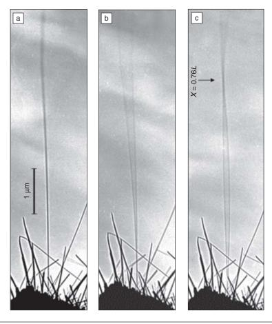
Figure 3. Nanotube response to resonant alternating applied potentials. (a) In the absence of a potential, the nanotube tip (length  $L=6.25~\mu m$ , diameter D=14.5~nm) vibrated slightly because of thermal effects. (b) Resonant excitation of the fundamental mode of vibration (frequency  $v_1=0.53~hm$ ); the shape corresponds closely to that expected for a cantilevered uniform beam. (c) Resonant excitation of the second harmonic (frequency  $v_2=3.01~hm$ ).
