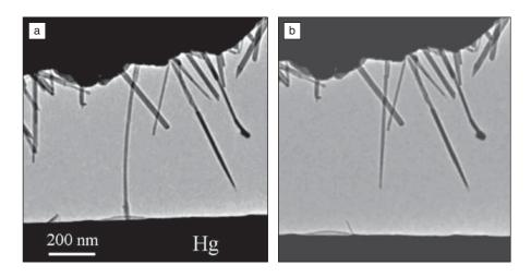
Figure 5. In situ observation of electric transport through single carbon nanotubes. (a) Applied voltage V=0.1 V, current  $I=7.3~\mu A$ , the resistance of the carbon  $R=12.7~k\Omega$  which corresponds to a conductance  $G=(12.7~k\Omega)^{-1}=1.02~G_0$  where  $G_0$  is the quantized conductance of a single conduction channel. (b) After applying a 4 V voltage, the nanotube was broken; the break occurred at the contact of the nanotube and the Hg.
