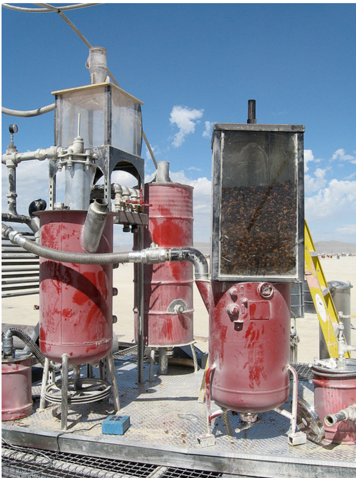
Figure 9: Gasification equipment on board Mechabolic .
