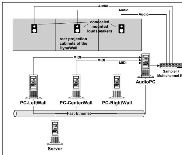
Figure 4: Hardware setup of the DynaWall
