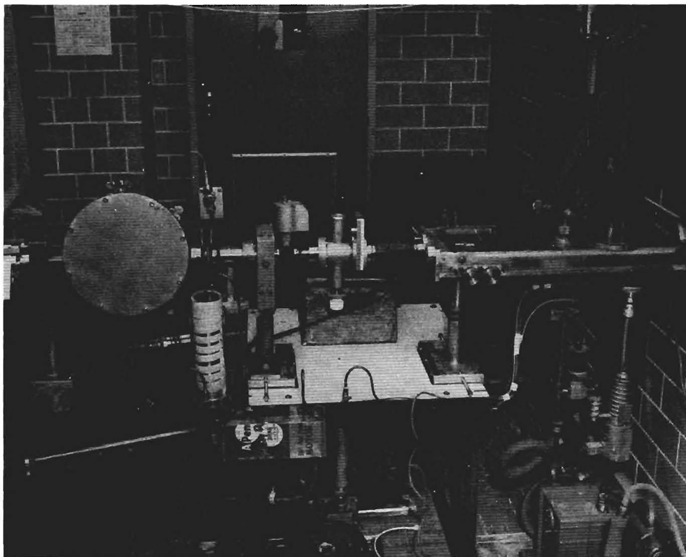
Figure 3. Exterior View of Electrostatic Analyzer and Collision Chamber.
