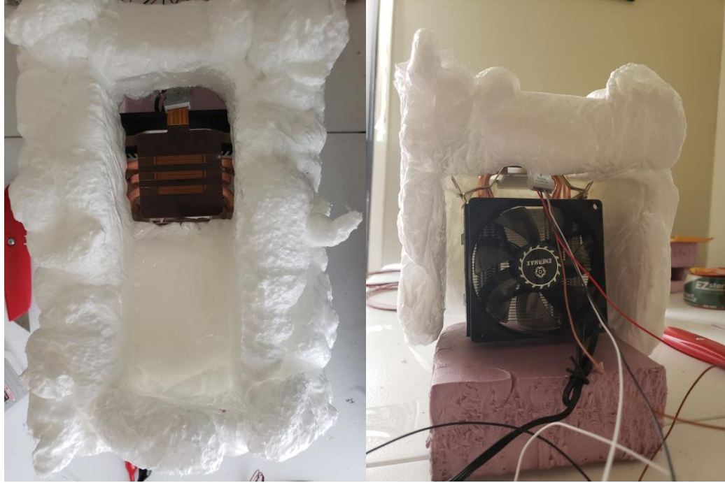
Figure 20 – Foam insulation setup. Left: Top view, Right: Cooler/back view
