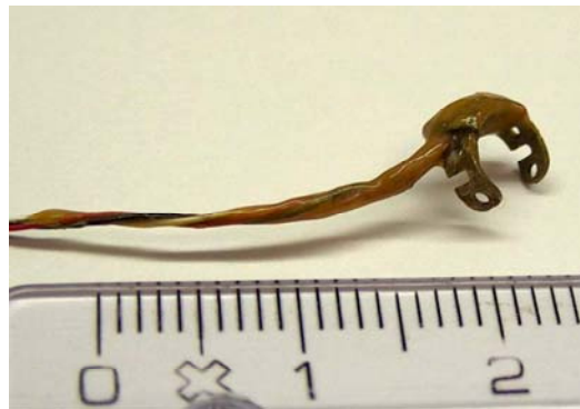
Figure 4.10. Photograph of a c-ring force transducer (scale in mm).
