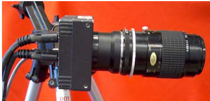
Figure 4.12 Photograph of a Basler A504K high speed camera
