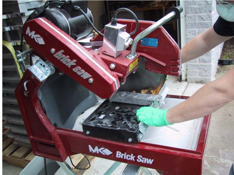
Figure 3.2: Water-Cooled Masonry Saw Utilized in Coupon Harvesting
