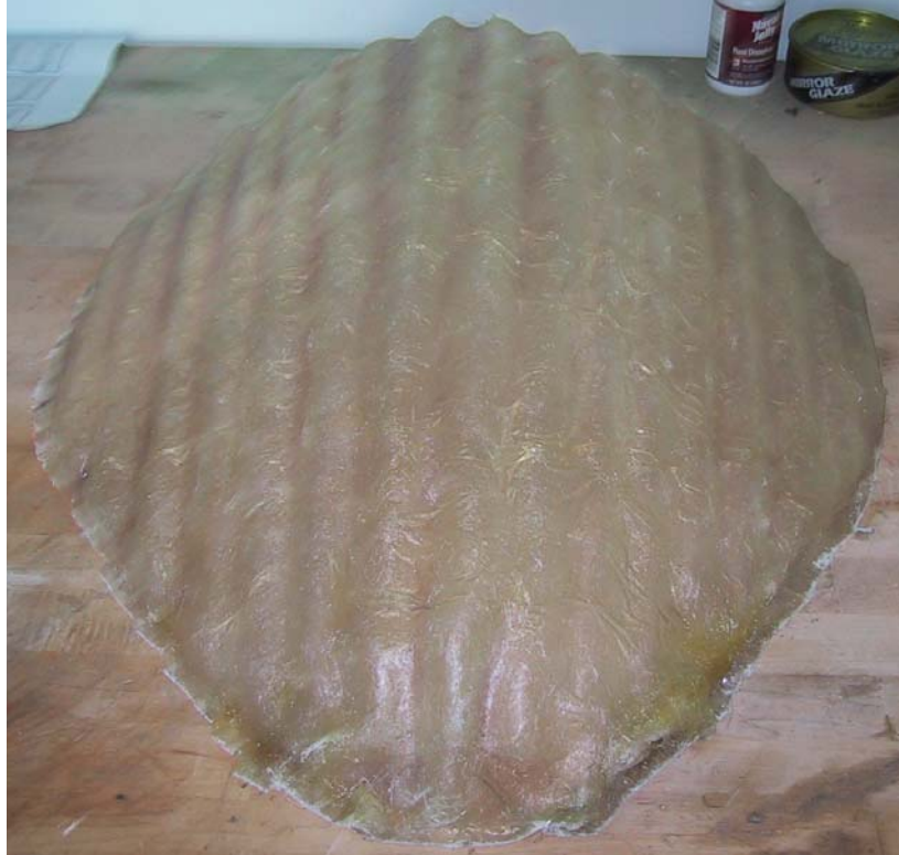
Figure 6.11: Synthetic Carapace 2 Fully Cured and Removed from the Mold
