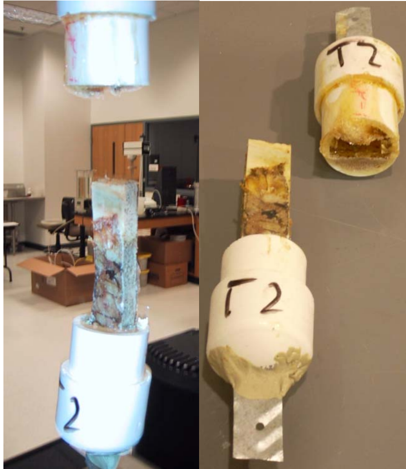
Figure 4.19: Unsuccessful Test due to Failure of the Bone-Epoxy Interface
