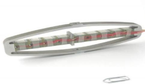
Figure 6 - Amplified Piezoelectric Actuator [76]
