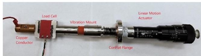
Figure 28 - Contact bolted to linear motion actuator
