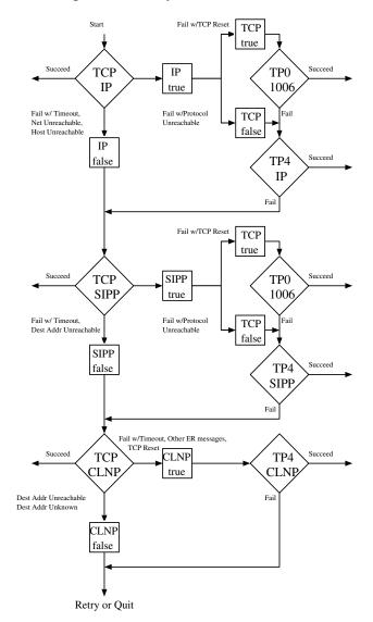
Figure 5: Protocol Discovery Algorithm
