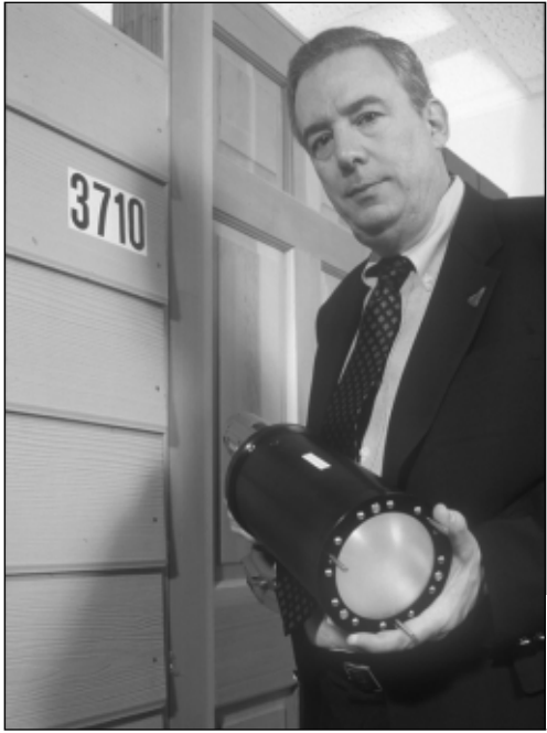
Researcher Gene Greneker demonstrates the RADAR flashlight.
