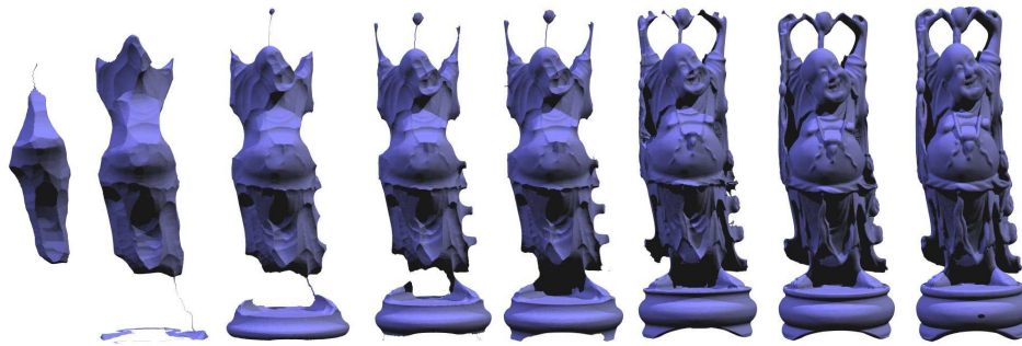
Fig. 5. Snapshots of the carving procedure for \tau = 20 . Note that all surfaces throughout the process are connected and have genus between 0 and 2.
