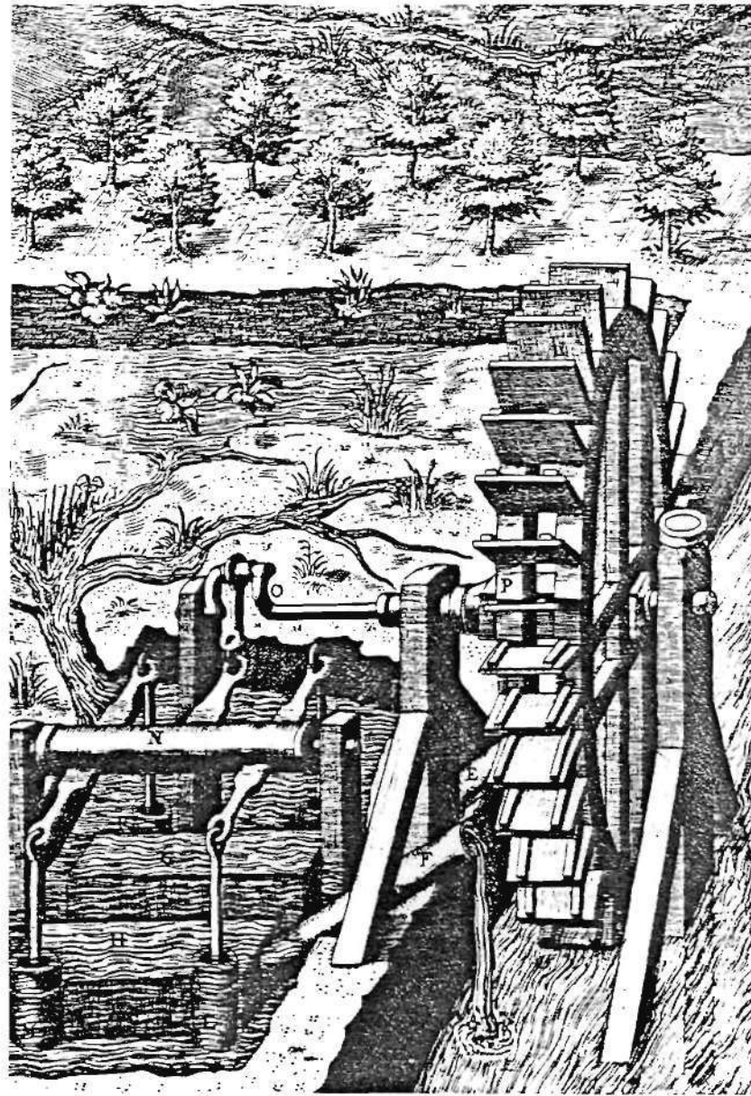
Water-powered piston force pumps using crankshaft and rocking beam, Ramelli, 1588
