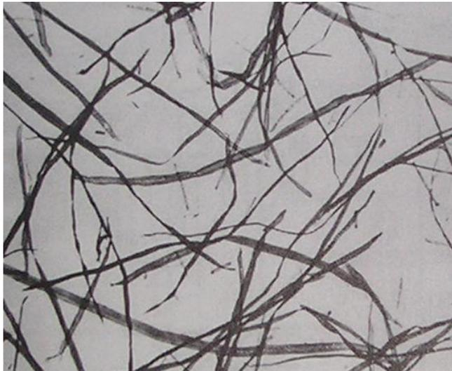
**Figure 2.2.2** –Micrograph of softwood fibers magnified 200X<sup>5</sup>
