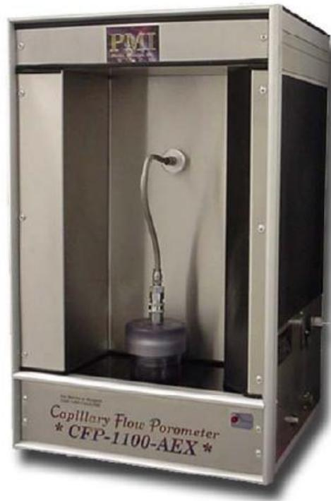
**Figure 3.2.1** – Picture of Porous Materials Inc. Porometer<sup>17</sup>
