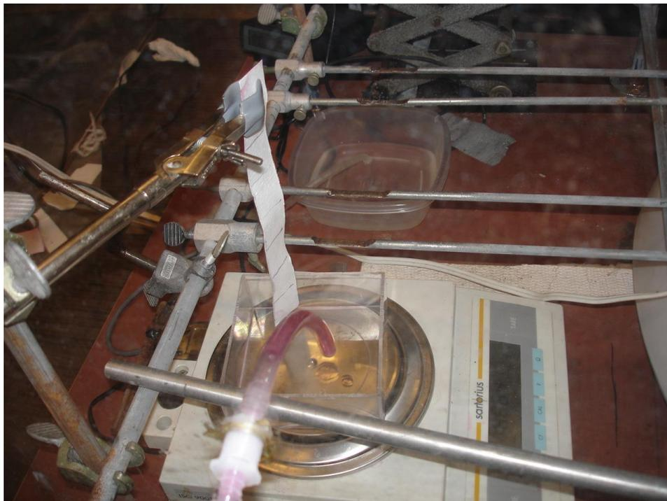
**Figure 3.3.1** - View of balance, siphon, and reservoir
