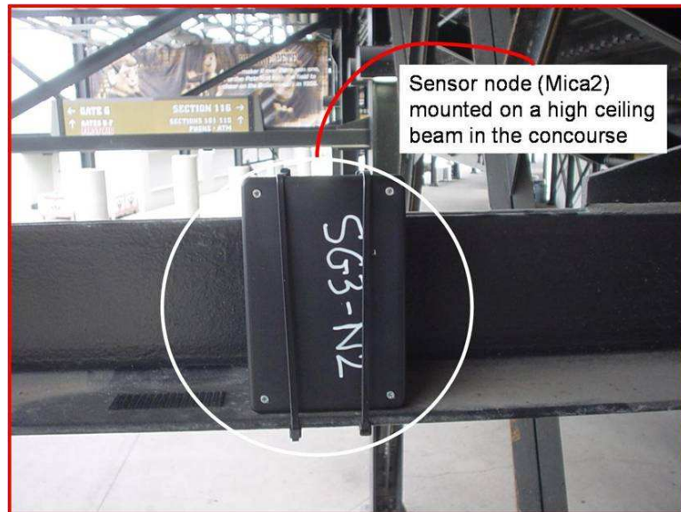
Figure 2: A Mica2 wireless sensor mote inside an enclosure that is strapped to a steel girder of the stadium.
