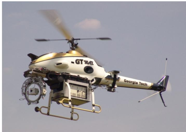
**Figure 1. GeorgiaTech GTMax UAV – Potential test vehicle for approach developed here**
