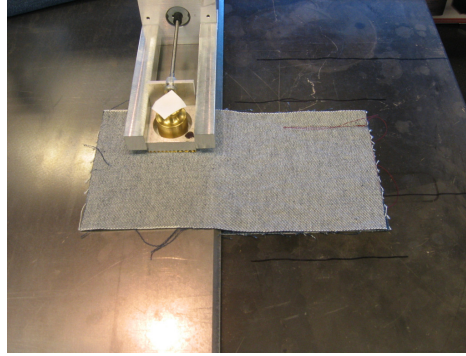
Figure 47 Two sheets of fabric were sewn together 3 inches along an edge as would be done on a standard seam. The top sheet was translated by the top dog while the bottom sheet was held in place by the bottom dog.
