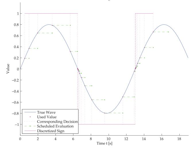
Fig. 4. The action 'checkSineWaveSign' evaluates the resource 'sineWaveValue' to evaluate its sign, which is stored as +1 or -1 in the resource 'sineWaveSign'. By dynamically computing  $\Delta t$ , update times focus on the region where the sinewave crosses zero, leading to increased precision while keeping the number of evaluations low.
