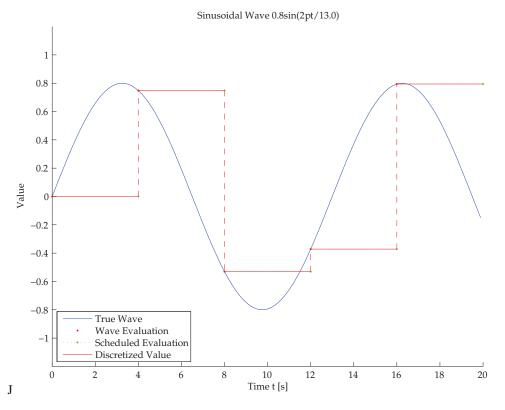
Fig. 5. Comparing the true value of a sine wave to a the value of the resource 'sine Wave Value' when action 'update Sine Wave Value' is called every 4.00s.
