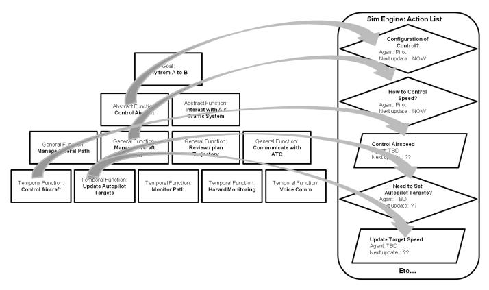
Fig. 3. Translating the work model into the action list used by the simulation engine (figure adapted from [8])
