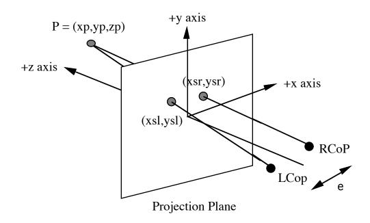
Figure 2. Stereoscopic Perspective Projection
