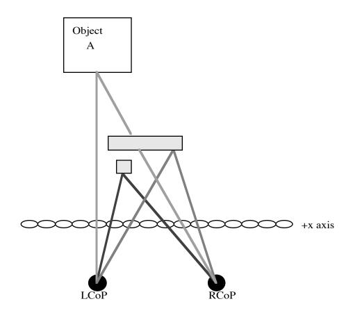
Figure 4b. Object A is blocked in the right-eye view and should <u>not</u> appear
