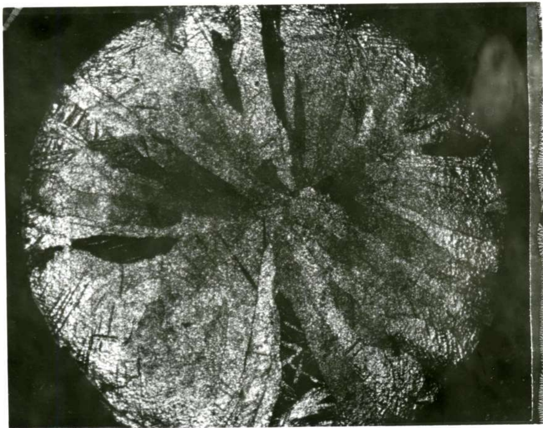
Figure 24. Photograph of the Zinc Metal as Received. x10
