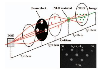
Fig. 1. (Color online) Schematic of the compact optical correlator using a DOE beam splitter. The DOE is a 2D phase grating with 40  $\mu m$  periods in both directions. Images for processing are inserted into the beam paths of the three (±1,±1) order beams picked by the beam block. The inset shows the ten generated THG beams captured by an Si CCD camera. The center THG beam,  $\mathbf{k}_1 + \mathbf{k}_2 + \mathbf{k}_3$ , is used for correlation.
