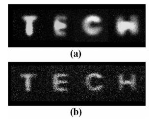
Fig. 2. Frequency converted letters taken at the image plane with an Si CCD camera. Using points to simulate the delta function in beams 1 and 3, images were encoded in beam 2 at frequency  $\omega$  and frequency converted to  $3\omega$  using THG in an organic film. Better resolution was obtained when the points better approximated the delta function. Diameter of the points: (a) 1.0 mm, (b) 0.5 mm.
