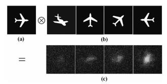
Fig. 4. Inverted target image (a) in beam 1 and input images (b) in beam 2 used for the correlation experiment. The corresponding correlation results are shown in (c).  $\otimes$  denotes convolution.
