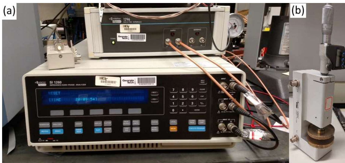
Figure 24 – (a) A Solartron 1260 analyzer with a Solartron 1296 Dielectric Interface (Solartron Analytical, Farnborough, Hampshire, U.K.) and (b) a parallel plate setup.
