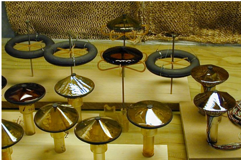
Several ballute wind tunnel models of various configurations were constructed and tested at NASA Langley.
