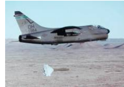
Ballutes for munitions deceleration
